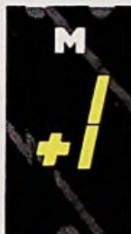
MAN 83 Common Anode; Overflow ( \pm 1 )
