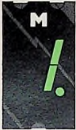
MAN 51 Common Anode; Right Hand Decimal
