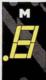
MAN 82 Common Anode; Left Hand Decimal
