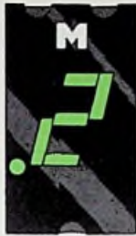
MAN 52 Common Anode; Left Hand Decimal
