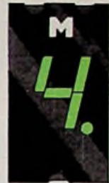
MAN 54 Common Cathode; Right Hand Decimal
