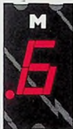
MAN 72 Common Anode; Left Hand Decimal
