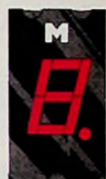
MAN 74 Common Cathode; Right Hand Decimal
