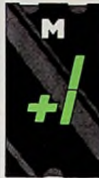
MAN 53 Common Anode; Overflow ( \pm 1 )
